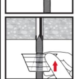
**Hilti HVU2 adhesive anchor capsule for anchor fastening in concrete**
